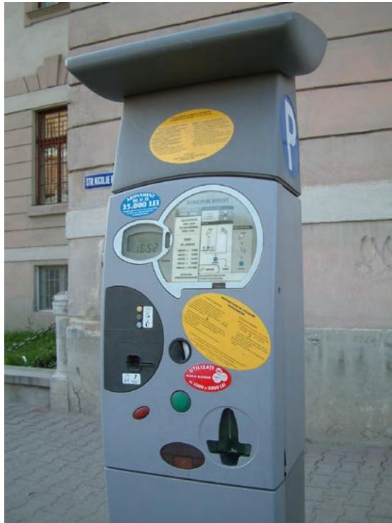
Figure 67 Solar-powered electronic parking meter for on-street parking.
