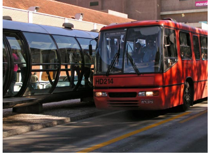
Figure 55 ▲ A high level platform like this one in Curitiba reduces boarding time, and so bus travel time.
