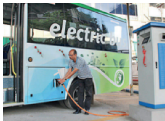
Figure 5 | Plug-in charging of an e-bus in India
