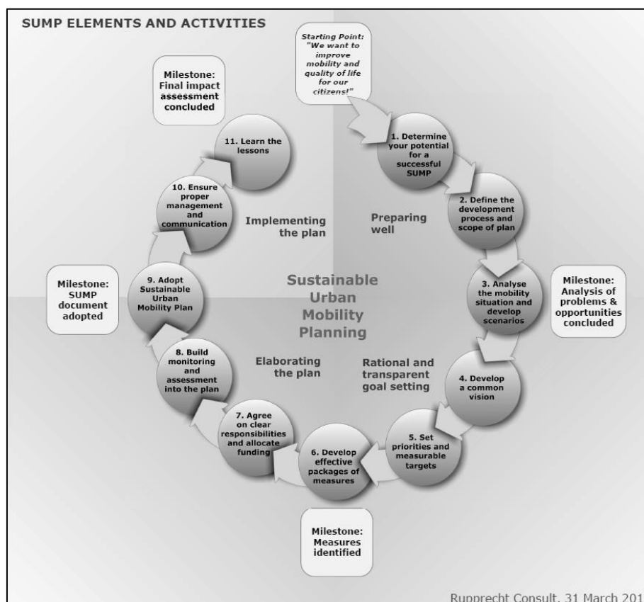
Fig. 3: Essential elements of the process of sustainable urban mobility planning shown as a cycle 11
