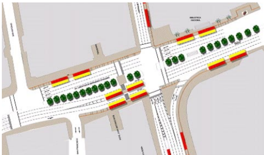
Fig. 5 Schematic of Transfer Station in Transantiago Plan. source: http://www.transantiago.cl
