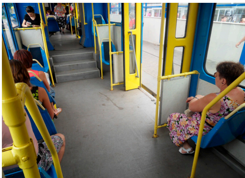
Figure 53: Tram modernisation is often a cost-efficient alternative to the procurement of new vehicles. The figure shows a refurbished tram with level-access entry operating at a Kiev tram system. © Mathias Merforth 2012
