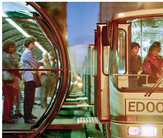
Fig. 51 and 52 The entry ramps used in Curitiba (left photo) and Quito (photo below) help to speed passenger boarding and alighting as well as improve passenger safety. Left photo courtesy of Volvo Photo below by Lloyd Wright
