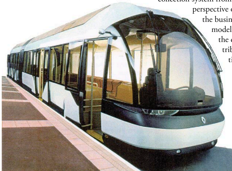
Fig. 68 The vehicle in this photo is a bus and not a light rail vehicle. The advent of modern, rail-like vehicles is helping to transform the image of buses as public transport.
