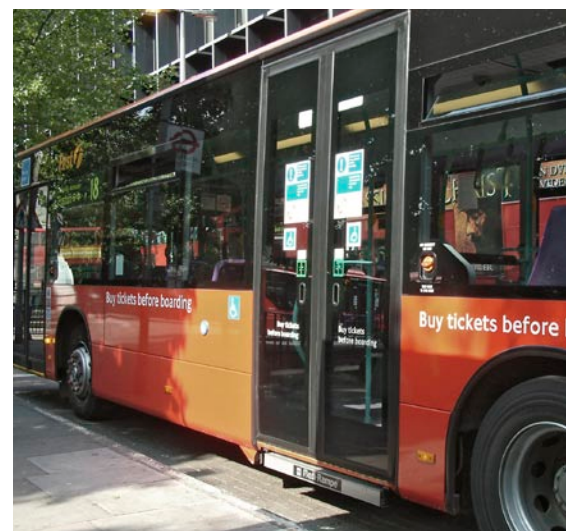
Fig. 65 Low-floor vehicles are increasingly popular in North America and Western Europe but do not always meet the needs of BRT systems in developing cities, where level boarding may be more appropriate.
