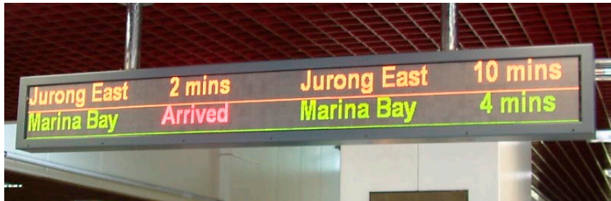
Fig. 26 Placing real-time information displays at station entrances allows customers to make key decisions about their journey.
