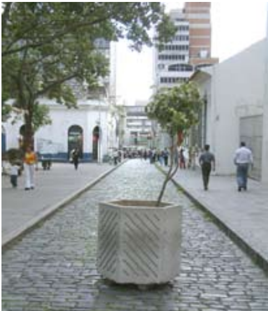
Fig. 127 A planter, as shown here in Caracas (Venezuela), can be both aesthetically pleasing and provide a semi-permanent barrier to vehicle entry.
