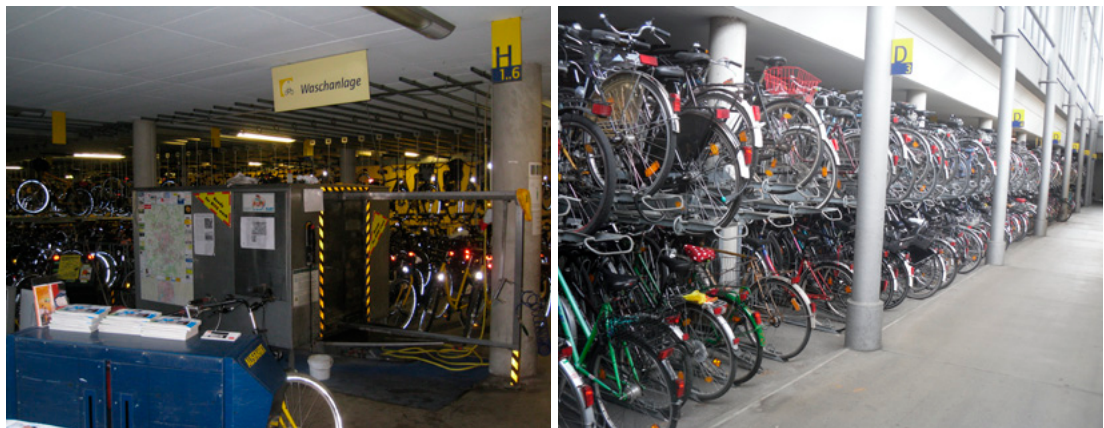
Figures 29 Bicycle station – Bicycle wash (left) and bicycle parking in two levels (right).
