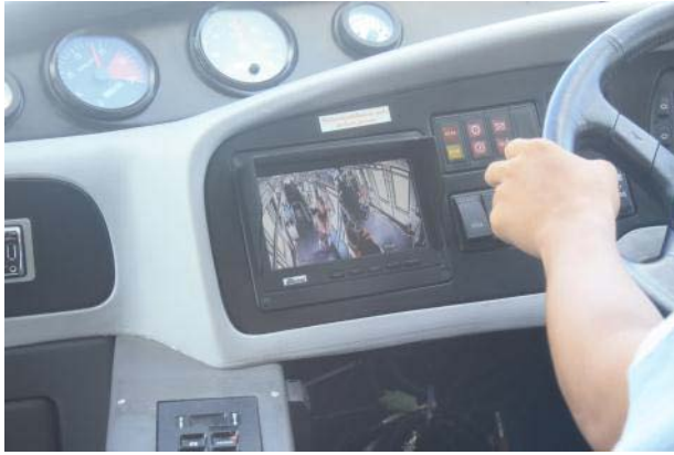
Figure 19: Display at the driver showing the passengers in the bus and also to manually control the opening and closing of the door.
