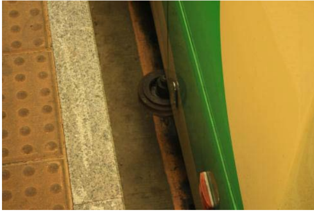
Figure 16: Mechanical Wheel for guiding the BRT bus into the bus bay.
