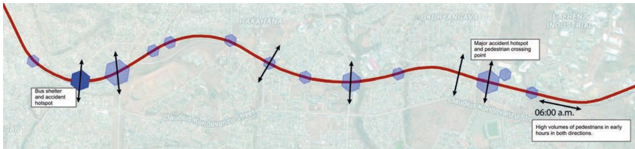
Fig. 11: Accident hotspots - A section of Monte Christo Road in Windhoek showing the interlinkage between accident hotspots and pedestrian crossings. Source: GIZ Transport Namibia 2016
