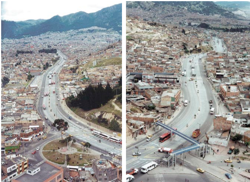
Fig. 3 Corridors in Bogotá where the TransMilenio system operates: Many developing cities, even though increasingly traffic-saturated, retain a corridor orientation which is conducive to Mass Rapid Transit.
