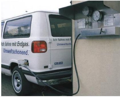
Fig. 2-1 Fast-filling at Ruhrgas in Dorsten
