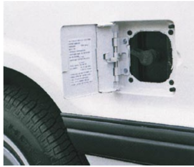
Fig. 2-2 Tank opening at the vehicle
