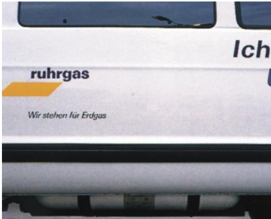
Fig. 2-5 Side view: High-pressure tanks under the vehicle Ruhrgas AG
