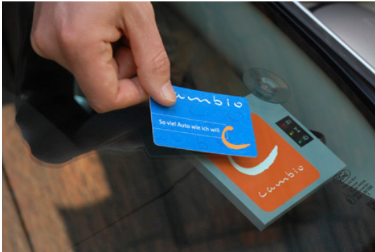
Figure 8: RFID card access to a carsharing vehicle. © Website Bundesverband CarSharing e.V.
