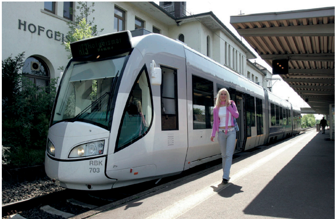
Figure 13 RegioTram as a dual-system or hybrid vehicle used on both city light-rail and regional rail lines within the Nordhessischer Verkehrsverbund (NVV).
