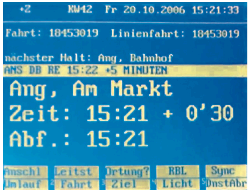
Figure 47 Details of a delayed regional express service (ANS(chluss)DB RE) displayed on the on-board computer of a public transport vehicle.
