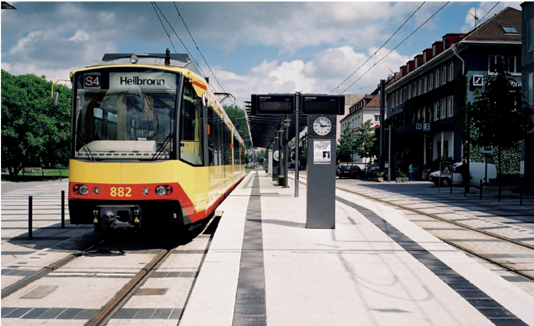
Figure 12 Electric dual-system light-rail coach operating a scheduled service within the Karlsruher Verkehrsverbund (KVV).
