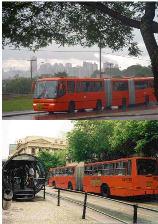
Figure IV-12: Curitiba: articulated and bi-articulated buses operating on exclusive busways provide very high capacity and reliability
