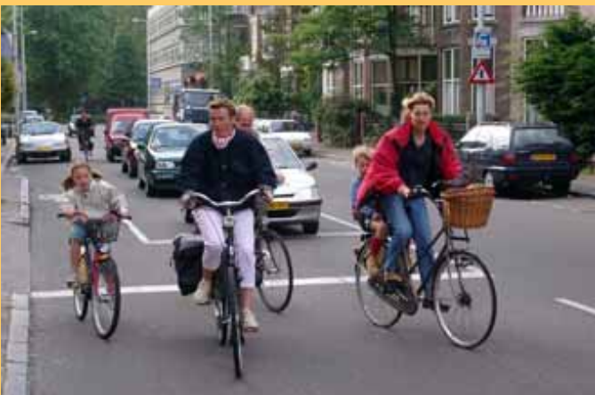
An advanced stop line for cyclists makes them more visible and provides them with right of way (Utrecht, The Netherlands)
