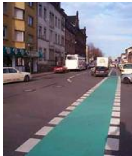
A painted stripe in Offenburg , Germany , gives cyclists a clear space through the intersection
