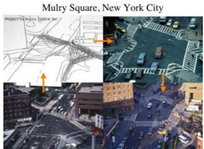
Tracking survey used as an inter-section redesign tool, Mulry Square, New York, USA
