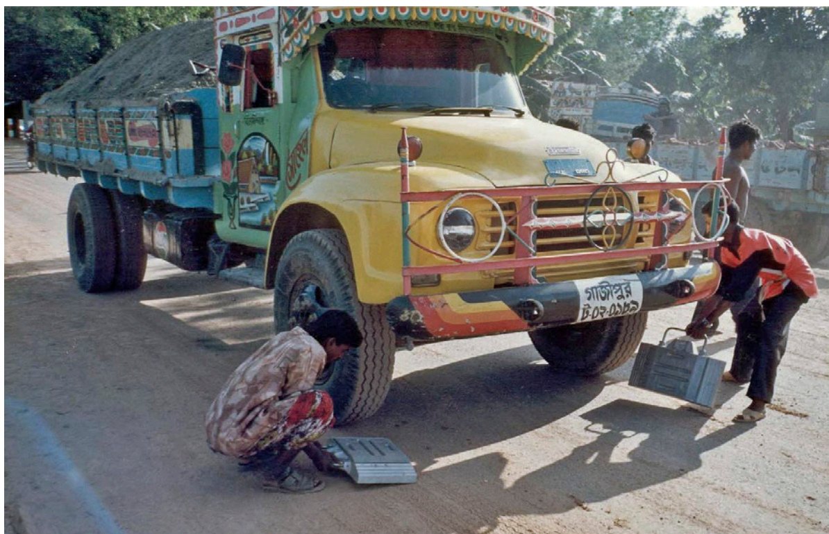
Figure 26: In order to control overloading, traffic police in Tangail district, Bangladesh use mobile measuring units ('mobile courts'). © Rainer Kuhnle
