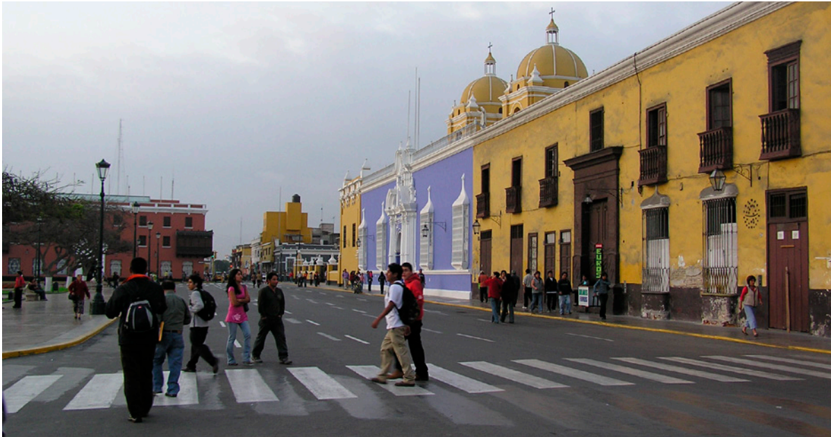
Figure 16: Zebra crossings are a useful tool, but only if adequate speed restrictions are enforced and crossings are respected by motorists. (This example of a zebra crossing in Peru is not good practice. Where more than two lanes are to be crossed there should be a central refuge for pedestrians to stop in safety while waiting for a gap in traffic.)
