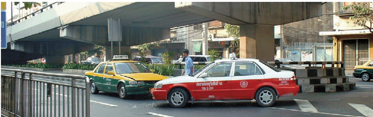
Figure 9: A combination of low cost measures such as better channelisation, medians and traffic signs, for example – could have averted this accident in Bangkok, Thailand, which was caused by confusion surrounding a contra-flow bus lane.
