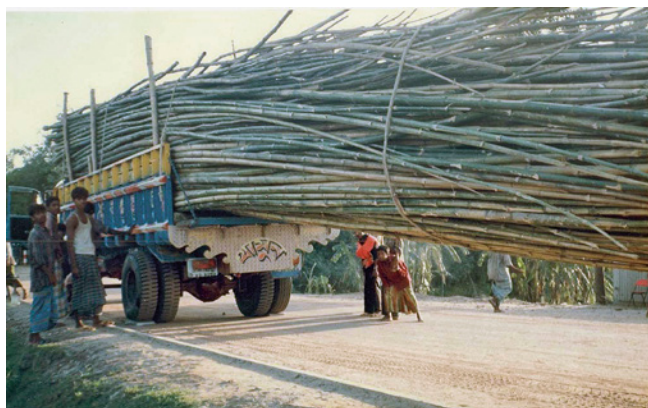
Figures 24 and 25: Overloading is a major cause of crashes. The front wheels of a truck loaded with bamboo trunks in Bangladesh (top) barely touch the ground, while a grossly overloaded truck in Amritsar, Punjab, India is a serious hazard.
