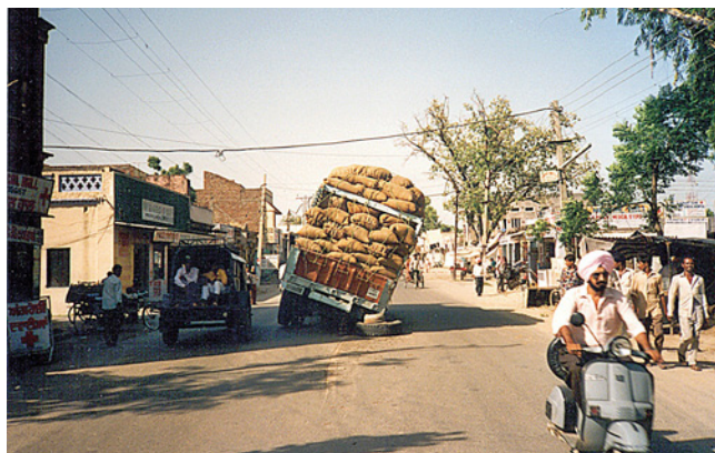
Figures 24 and 25: Overloading is a major cause of crashes. The front wheels of a truck loaded with bamboo trunks in Bangladesh (top) barely touch the ground, while a grossly overloaded truck in Amritsar, Punjab, India is a serious hazard.
